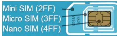
Figure 2: SIM Card Size Formats [Orm09]
